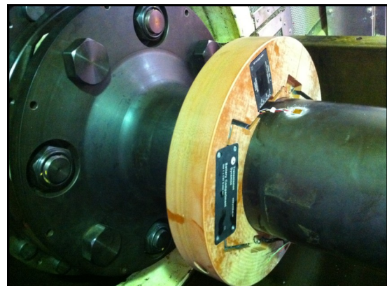
Above: Radio Microlog torque monitoring installation.
